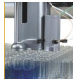
Inject, collect fractions and re-inject on the same bed.
