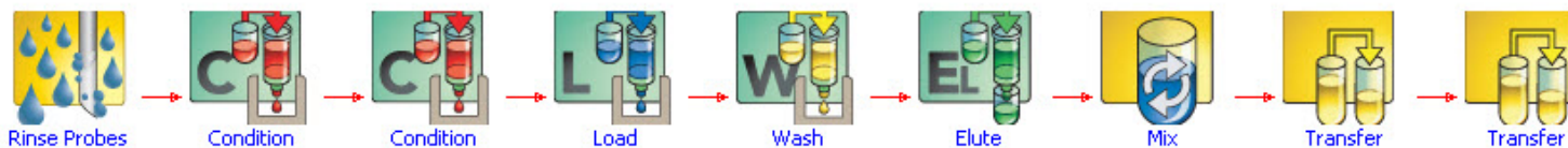
Figure 4. TRILUTION® LH Iso-Alpha Acid Solid Phase Extraction Method Using the GX-271 ASPEC™ with Dual 406 Syringe Pump
